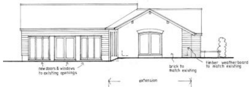
north west elevation
